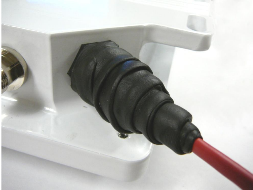
Figure 7.6.1: Properly taped Ethernet adapter
