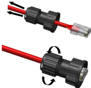
Figure 2.2.4: Tightening the End Cap
