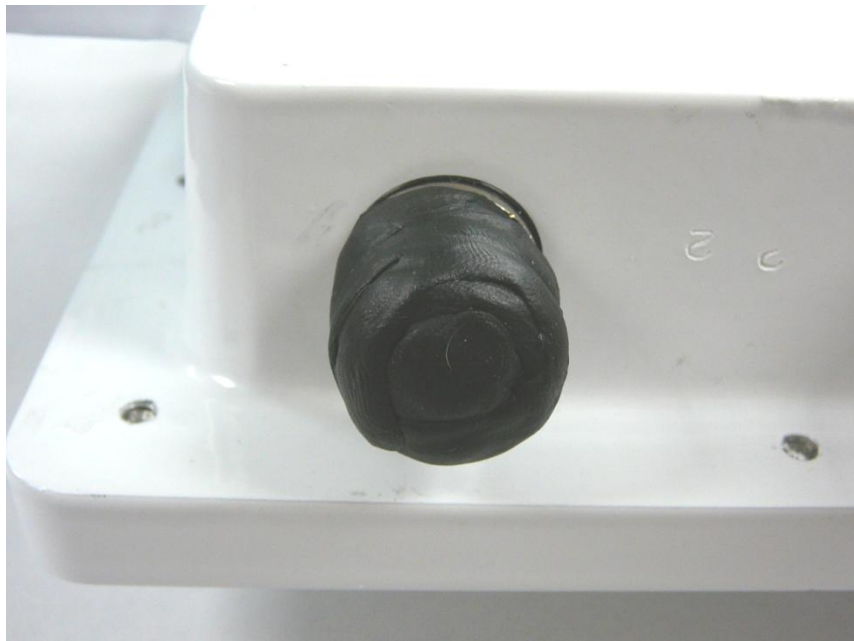
Figure 7.6.2: Properly taped external antenna port.
